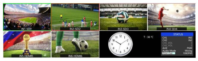
The lower right corner display of the menu and status information. The CH1, CH2 are the channel selection of the 2 audio sources for audio mixer. There is a real-time Digital clock/Analog clock displayed beside the menu.
