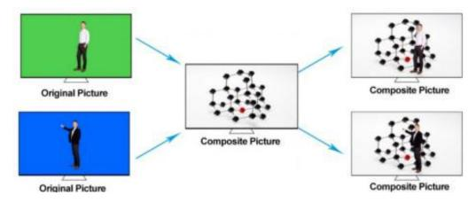
1) Switching a video with blue or green background to PVW window, and turn on the Chroma Key. Then enter into the Key menu to configure the value of Chroma Key. Using CUT, AUTO, or T-Bar to switch the image to overlay in the PGM window.
