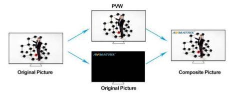
When turn on the Luma Key, all of the black areas defined by the luminance in the video signal will be made transparent so that the background can be revealed underneath. Therefore, the final composition does not retain any black from the graphic because all of the black parts have been cut out of the image. This function is often used for subtitle overlay of virtual studio.
