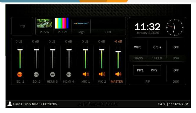
The information of user name, working time, USB connection, CPU working temperature, system time keeps displaying in the bottom of the Status/Menu page.
